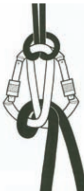
33 The Gegenlaufesperre This hitch offers inconsistent performance and reliability.
