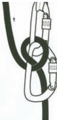
40e Improper braking method with the carabiner wrap belay The correct side of the rope being used, but it will get pinched by the load- bearing side.
