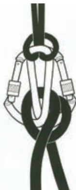
32 Gleichlaufesperre failure The hitch can shift into something that resembles the Münter hitch, and the rope will not lock up.
