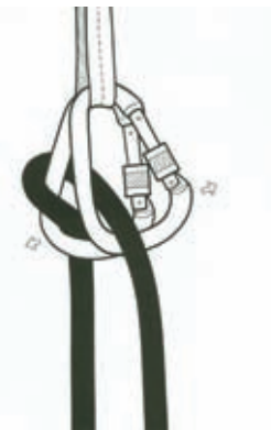
26b Garda failure - method 1 The rope can slip as the HMS carabiners pivot apart.
