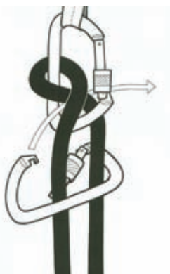
37b Setting up the C & F belay hitch - method 2 Clip the lower carabiner, as shown.
