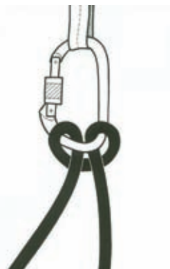
2b Girth hitch on a carabiner The right-hand side of the rope bears the load.
