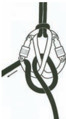
31d Re-clipping the Gleichlaufesperre Follow the transition from 31a to 31b to 31c to 31d and back to 31a.
