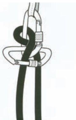
37c The C & F belay hitch with the gate opening downward Note that the load is on the left-hand side of the line.
