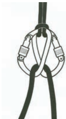
31c The Precursor belay Follow the transition from 31a to 31b to 31c to 31d and back to 31a.
