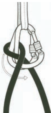
28a Garda failure - method 3 The tight wrapping the carabiner spines slips down.
