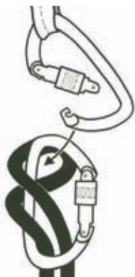
39b Setting up the carabiner wrap belay from scratch - step 2 Clip the lower carabiner, as shown.
